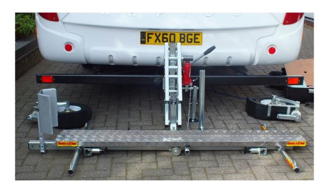
You jack it up take off the wheels and drop it down to put the scooter on then jack it back up and put the wheels on. I had a few alterations to do on the wheel clamps just to make it more secure and easy for me to put on and off.
